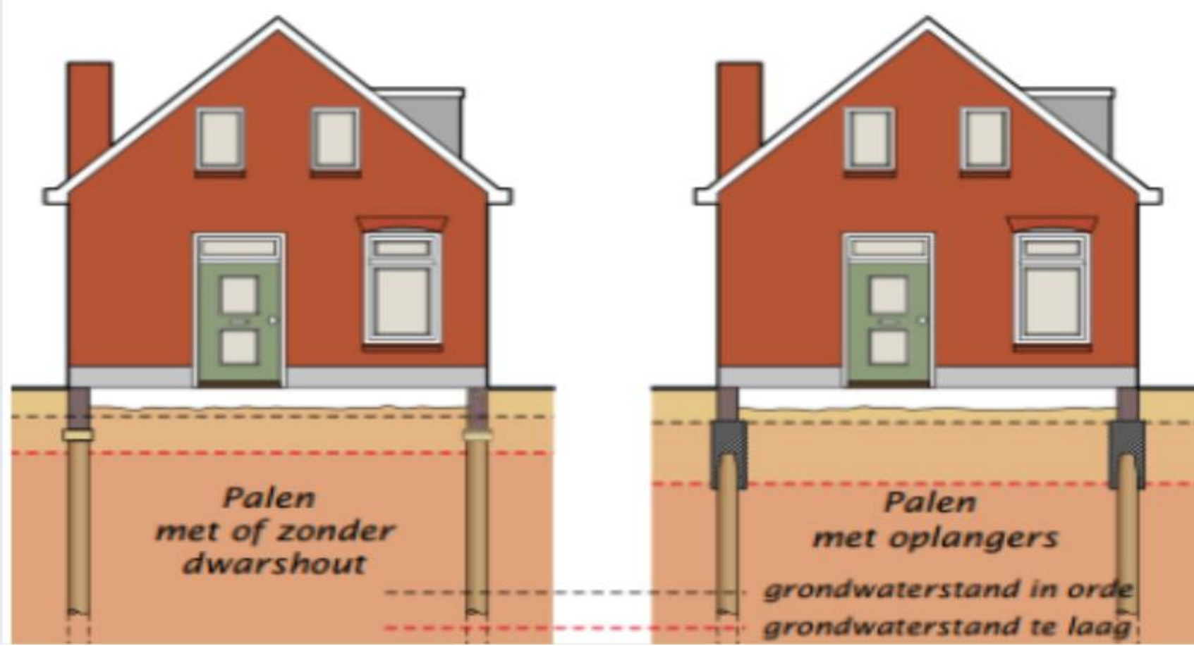
Application of upright pile extensions (in Dutch "opslagers") (image by Rioned)
