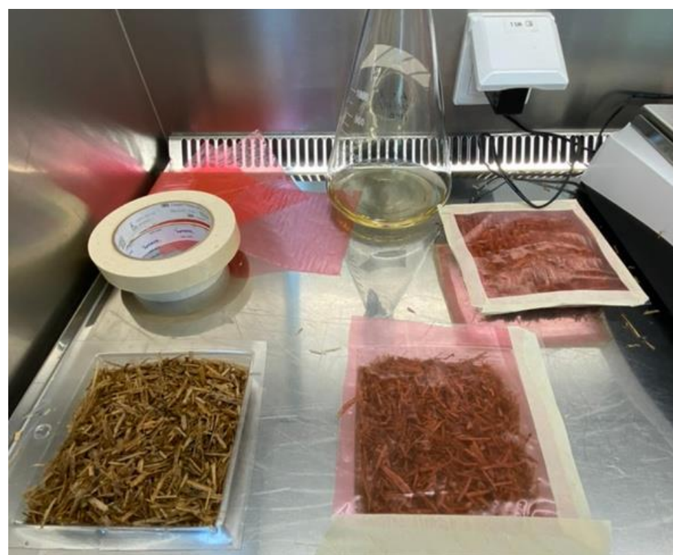
Figure 2: Liquid inoculum and mycelium moulding
