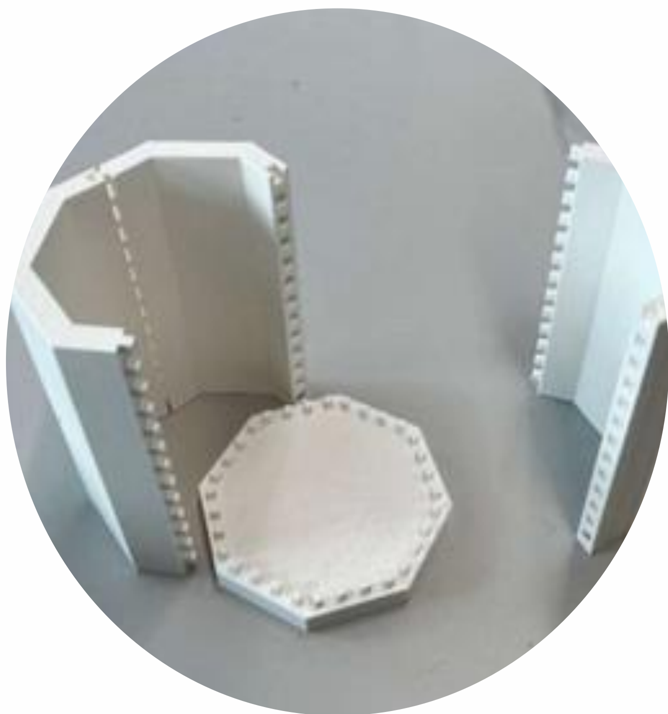
Octogen shape with puzzle joint system design.
