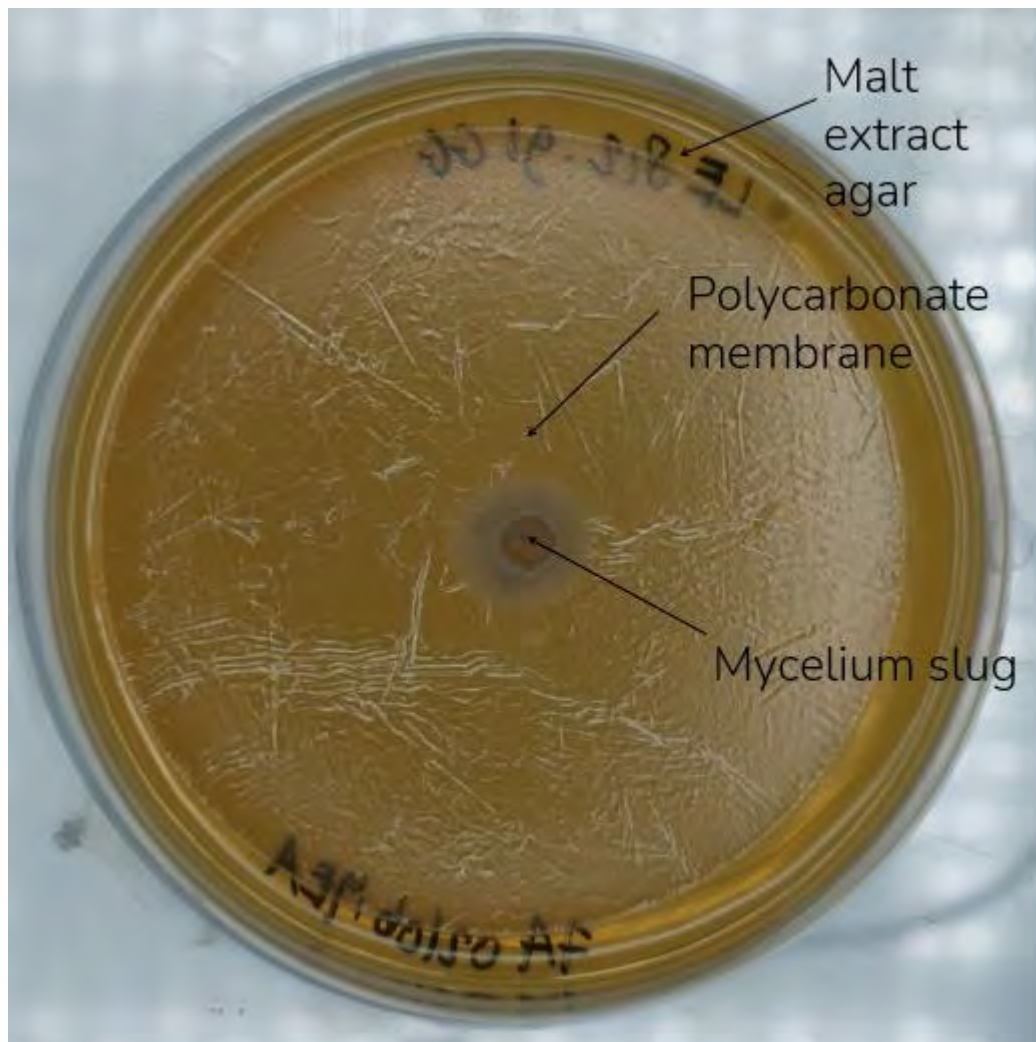
Figure 1 Lentinula Edodes (generation 7) growing on an agar plate with polycarbonate membrane.
