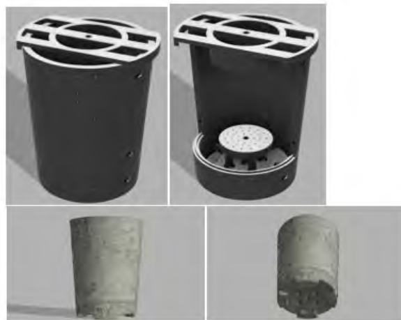
Figure 7 – Prototype mould design (above) with the visualization of the MBC pots (below), produced in SolidWorks
