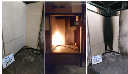
N-8010, Fire certificate according to EN13501 Class B-s1,d0
