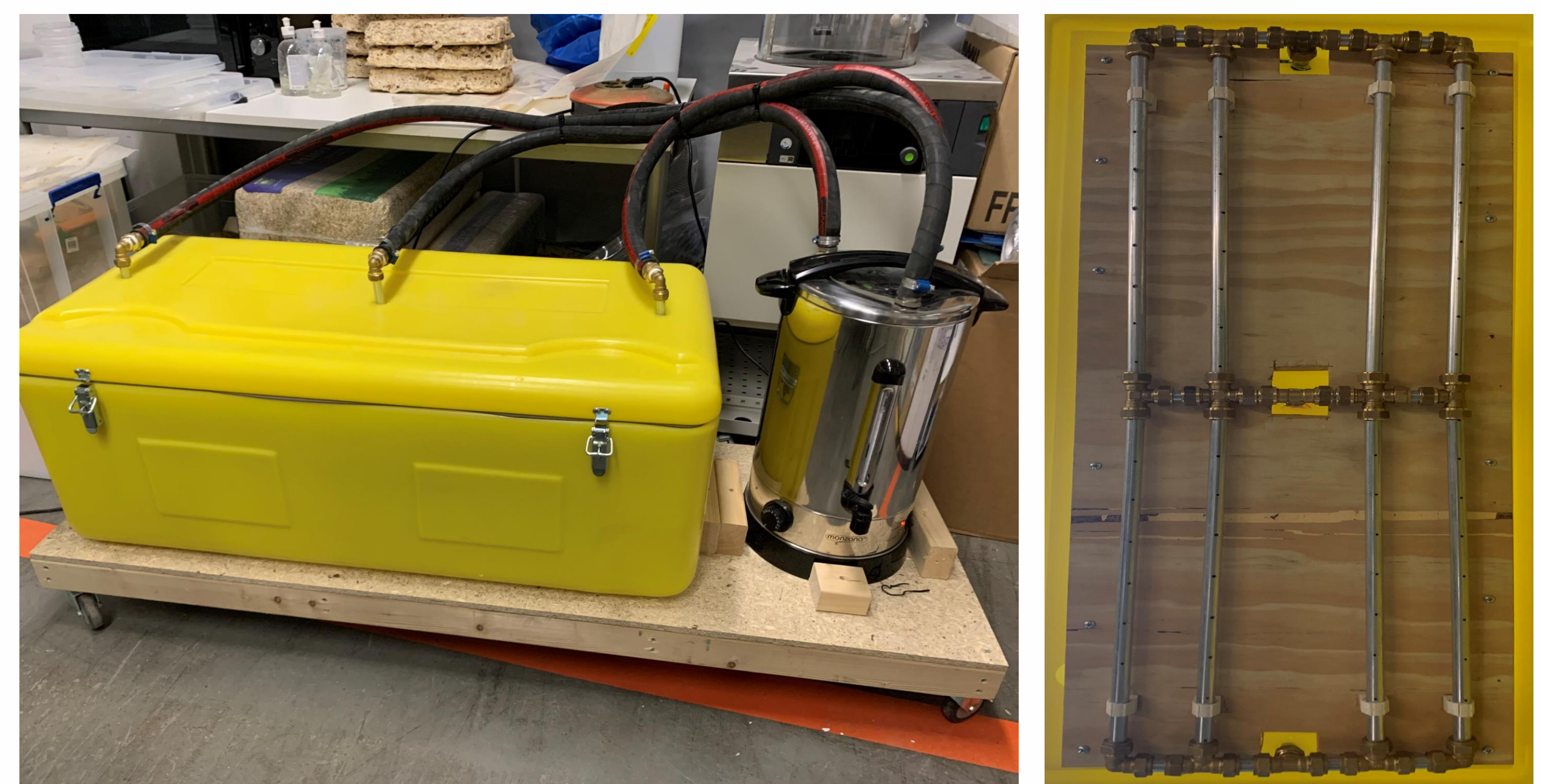
Images of the pasteurization setup and the pipe system that distributes the steam homogeneously
