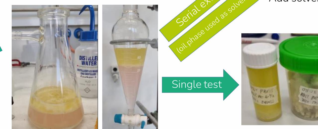
Separation of liquid phases
