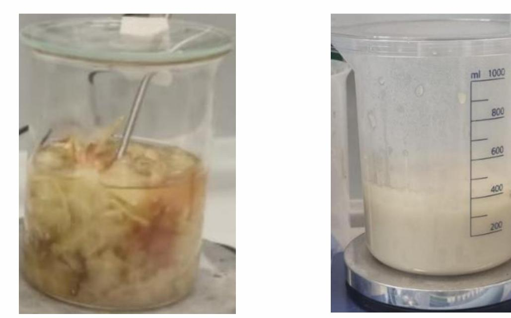
Two distinct experiments before filtering stage. Sharp contrast in visual aspect. Empirical observations and mass-balance calculations were used to improve and refine the methodology. The quality of the pulp and quantity of onions used were the most important parameters to ensure a good extraction result.
