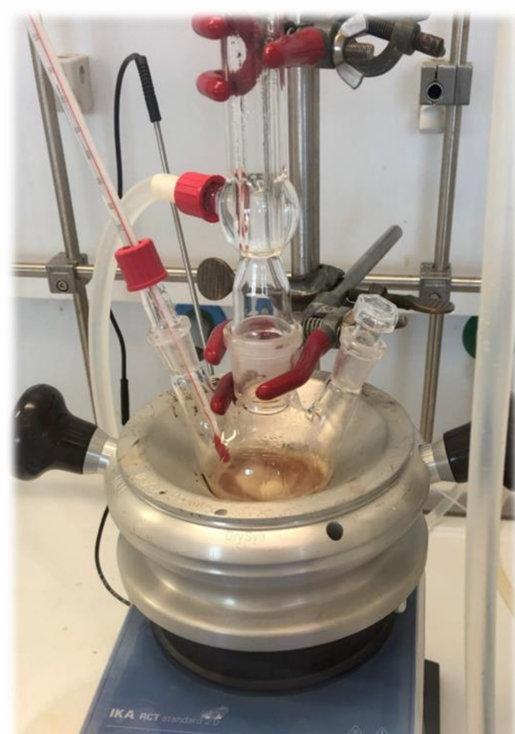
Figure 4: Photo of solvolysis setup.
